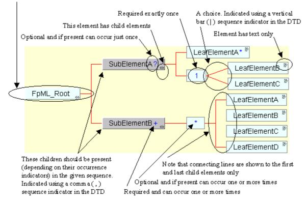
Figure 4.1: Graphical Representation of a DTD
