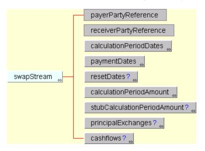
The structure of a swapStream is shown diagrammatically below:
