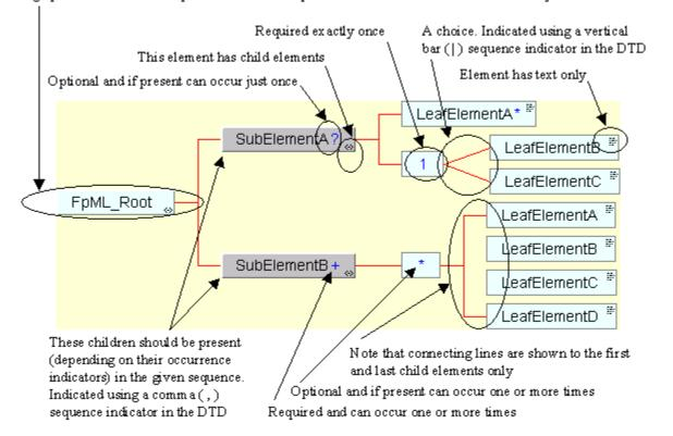
Figure 4.1: Graphical Representation of a DTD
